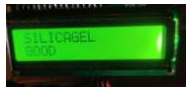
FIG.4 Silica in good condition
